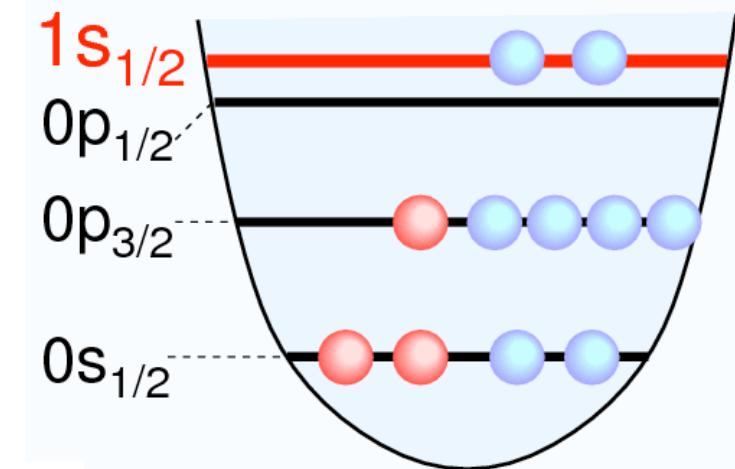
Deuteron structure in shell model is produced by 2p-2h states
