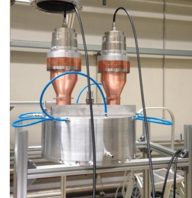
High power RF Coupler 200kW 100% duty cycle
