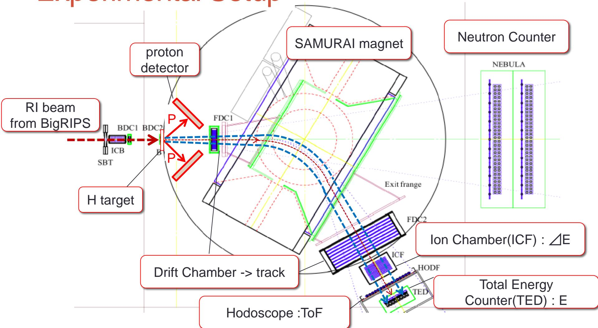
Charge(Z) and Mass(A) can be separated by  $B_p \Delta E$ -ToF(E)
