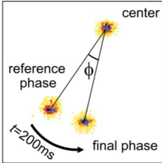
$$\begin{aligned} \varphi_g &= 2\pi \cdot f_g \cdot t \\ \varphi_m &= 2\pi \cdot f_m \cdot t \end{aligned} \quad \Rightarrow \quad \Delta\varphi = 2\pi \cdot (f_g - f_m) \cdot t$$
