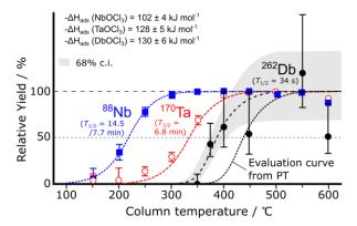
Fig.2 Comparative chromatograms for NbOCl<sub>3</sub>, TaOCl<sub>3</sub>, and DbOCl<sub>3</sub>. A curve for DbOCl3 evaluated from the Periodic Table is also shown. The gray area represents the 68% confidence interval (c.i.) of the DbOCl<sub>3</sub> yield.
