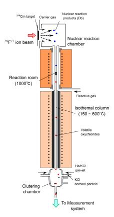
Fig.1. Schematic diagram of experimental setup
