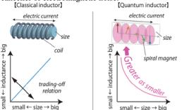
Fig.1 Comparison of classical and quantum inductors. The size (crosssection) dependence is totally different between two systems [3]. Non-reciprocal Pumping of Surface Acoustic Waves
