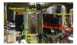
Fig2. Photograph of experimental setup at HIMAC. The plastic scintillators are installed both upstream and downstream of HypTPC as trigger counters. The silicon strip detectors are also installed both upstream and downstream of HypTPC as position reference detectors.
