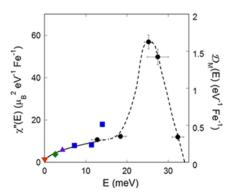
Fig. 2. Magnon density of states  $(\mathcal{D}_M(E))$  of YIG obtained by inelastic neutron scattering [4], which is proportional to imaginary part of dynamical spin susceptibility ( $\chi$ "(E)). The magnitude is one of the important factors for spin current power generation.
