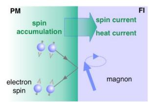
Fig.1 Schematic view of the spin Peltier effect. We consider spin and heat transports in a bilayer structure consisting of a paramagnetic metal (PM) and a ferromagnetic insulator (FI), where the electron spins in PI are coupled with the localized moments in FI via the magnetic interaction. The spin accumulation at the interface is found to be a driving force of spin and heat current.
