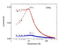
Fig. 2 Temperature dependence of magnetic susceptibility of UPtIn.
