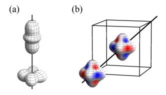
Fig. 2 (a) Non-magnetic state for ions aligned along a direction of a lattice axis. (b) Magnetic state for ions aligned along a diagonal direction.
