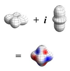
Fig. 1 Magnetic state composed of non-magnetic states with different shape of electron distribution. In the red and blue areas, the axes of the circulating currents are in opposite directions and produce opposite magnetic fields.
