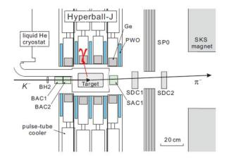
Fig. 1: The experimental setup of E13 [2]. The K beam is injected to the <sup>4</sup>He target. The incident K and the produced  $\pi$  are identified with the aerogel Cherenkov detectors BAC2 and SAC1. The gamma rays emitted from the target are detected with the Hyperball-J Ge detectors.
