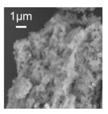
Fig. 2 SEM image of a typical particle of SSA. This particle looks sintered aggregate of numerous nanoparticles. In SSA, iron is contained in particles like this.
