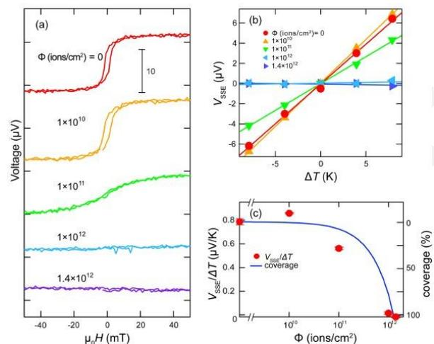
Fig.1-(a) Measured SSE voltage for the ion-irradiated samples with the fluence,  $\Phi=0, 1 \times 10^{10}, 1 \times 10^{11}, 1 \times 10^{12}$ , and  $1.4 \times 10^{12}$  ions/cm<sup>2</sup> (from top to bottom). The output signals as a function of applied magnetic fields. The temperature difference  $\Delta T$  between Pt and the substrate is fixed as 8 K.
