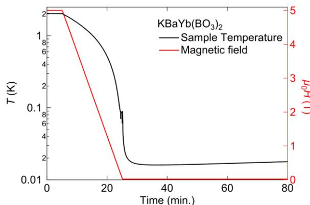
Fig. 2 Refrigeration test under nearly adiabatic conditions. The black and red lines are temperature (left axis) and external magnetic field (right axis), respectively. The final temperature is 22mK [6].
