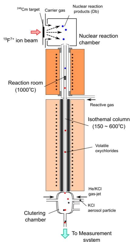
Fig.1. Schematic diagram of experimental setup
