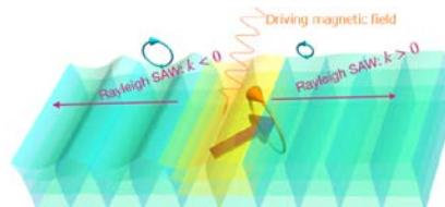
Fig.2 Schematic of the magnetic film [4]. The ring surrounding the thick arrow at the centre indicates the precessing magnetisation and the other rings at the back represent the rotation of surface atoms. In this figure, energy is dominantly channelled into SAWs propagating in the negative direction.
