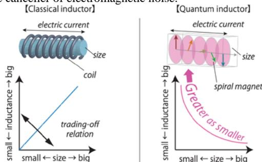
Fig.1 Comparison of classical and quantum inductors. The size (cross-section) dependence is totally different between two systems [3].
