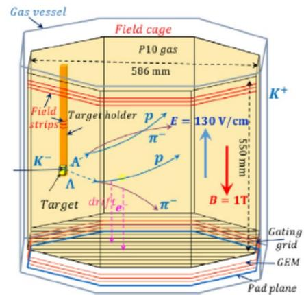
Fig1. Schematic view of HypTPC
