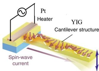
Fig.1 Schematic illustration of spin Seebeck mechanical force. When a part of a magnetic insulator is heated, a spin wave is excited and flows out of the part. A spin wave carries angular momentum. Relaxation of spin waves generates macroscopic mechanical torque and force due to the angular momentum transfer
