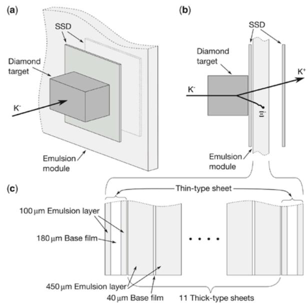
Fig. 1 Schematic view of the experimental setup around a diamond target. The target size is 50 mm (W) × 30 mm (H) × 30 mm (T).
