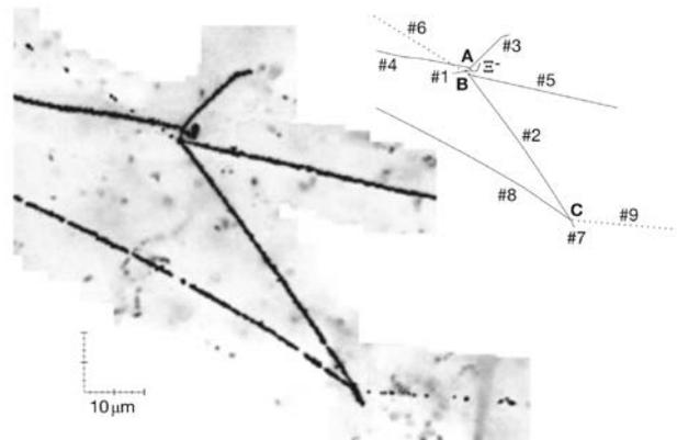
Fig. 2 A photograph of the MINO event and its schematic drawing.
