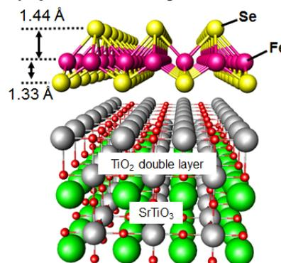
Fig.1 Asymmetrically optimized structure of single-layer FeSe on an oxide substrate, which was determined in this study. Se layer on the top of Fe layer becomes taller as compared to Se layer on the bottom.
