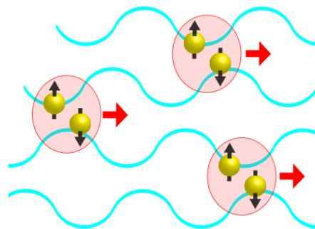
Fig.1 Schematic image of superconductivity. Electrons (yellow spheres) in material have a magnet-like character called electron spin (black arrow). A pair called Cooper pair is formed by directing this electron spin in antiparallel direction, and it flows like a wave, resulting superconducting state.
