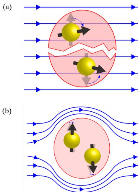
Fig.2 Cooper pairs' behaviours when magnetic field (blue solid line) is applied.
