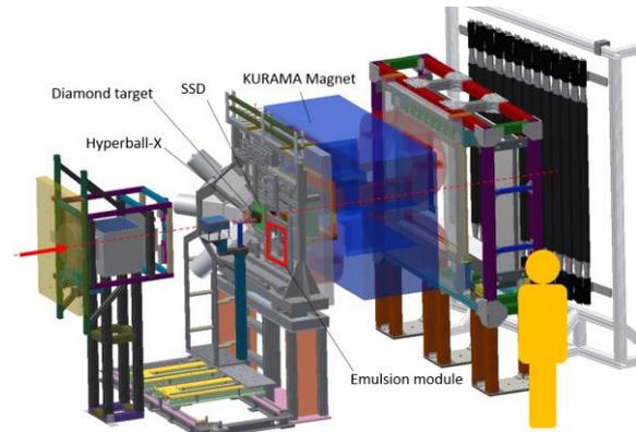
Fig.2 Experimental apparatus of J-PARC E07.
