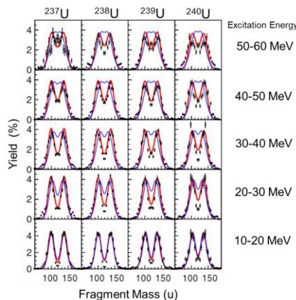
Fig.1 Fission-fragment mass distributions of uranium isotopes. The red and blue curves are the results of Langevin calculation with and without taking into account the multi-chance fission.
