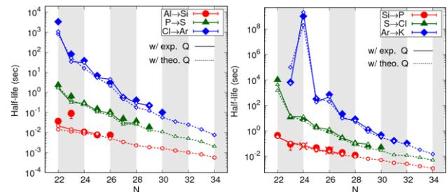
Fig. 2  $\beta$ -decay half-lives compared between experiment and theory. The filled symbols are experimental data, and the open symbols with the solid and the dashed lines stand for the calculated values using the experimental and calculated  $Q$  values, respectively.
