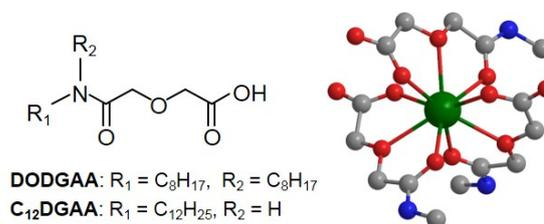
Fig. 1 Crystal structure of [La(DGAA)<sub>3</sub>]. Green = La<sup>3+</sup>; red = oxygen; blue = nitrogen; gray = carbon. Hydrogen atoms, alkyl chain, and H<sub>2</sub>O molecules are not shown for clarity.
