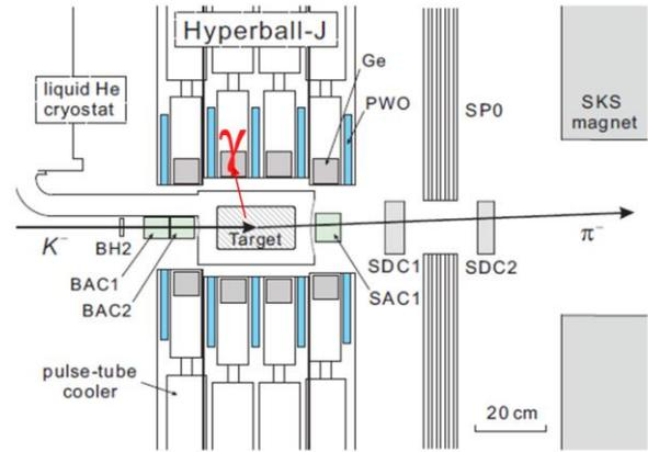
Fig. 1: The experimental setup of E13 [2]. The  $K^-$  beam is injected to the  ${}^4\text{He}$  target. The incident  $K^-$  and the produced  $\pi^-$  are identified with the aerogel Cherenkov detectors BAC2 and SAC1. The gamma rays emitted from the target are detected with the Hyperball-J Ge detectors.
