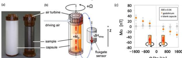
Fig.1 (a) Capsule (left) and Gd sample (right) used in the experiment. (b) Schematic figures corresponding to (a). (c) The magnetization of
