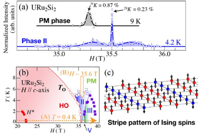
Fig. 1 (a)  $^{29}\text{Si}$  NMR spectra in the paramagnetic (PM) and the magnetic II phases, (b)  $T$ - $H$  phase diagram for  $\text{URu}_2\text{Si}_2$ , and (c) schematic spin structure in the II phase.
