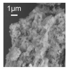
Fig. 2 SEM image of a typical particle of SSA. This particle looks sintered aggregate of numerous nanoparticles. In SSA, iron is contained in particles like this.
