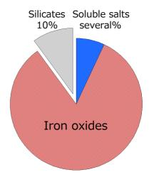
Fig. 1 Fractions of <sup>137</sup>Cs in sewage sludge ashes. The majority of <sup>137</sup>Cs is contained in iron oxides.
