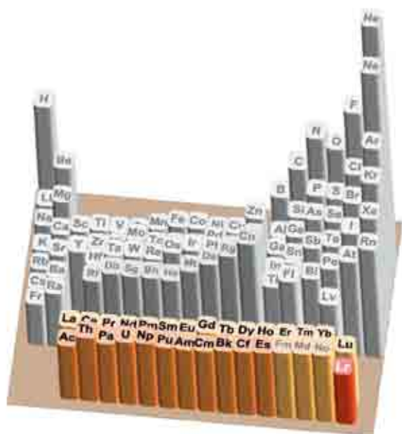
Fig.1 The first ionization potential of heavy lanthanides (●) and actinides including our present results for Lr (●: experimental, ○ estimated value, *: theoretical value for Lr [2])
