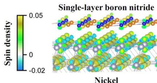
Fig. 2 Spatial distribution of the spin polarization at the single-layer hexagonal boron nitride/nickel interface in the energy region close to the Fermi level. The orange, blue, and gray spheres show boron, nitrogen, and nickel atoms, respectively. The sign and density of the spin polarization are represented by a gradational change in color (see the color bar on the left side).
