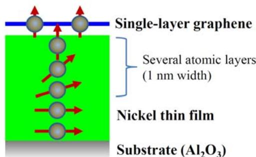
Fig. 1 Change of the stable spin direction in the region near the single-layer graphene/nickel interface. The arrows show the spin direction.
