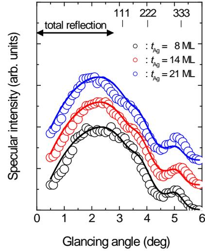
Fig. 1 TRHEPD rocking curves from the  $\text{Ag}_2\text{Pb}$  surfaces with the Ag film thicknesses ( $t_{\text{Ag}}$ ) of 8-21 ML. Open circles are the experimental curves and solid lines are the calculated ones using the optimum Pb heights.
