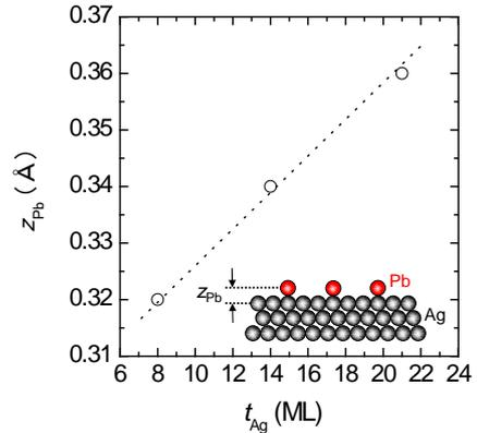
Fig. 2 Optimum Pb height ( $z_{\text{Pb}}$ ) from the underlying Ag layer in the  $\text{Ag}_2\text{Pb}$  surface alloy at each Ag film thickness ( $t_{\text{Ag}}$ ).
