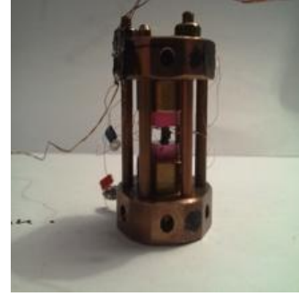
Fig. 1 The uniaxial pressure cell. The sample (black) is located between two clamps (red).
